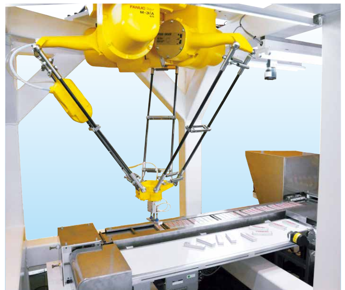
High speed arranging the foods by M-3iA/6S
