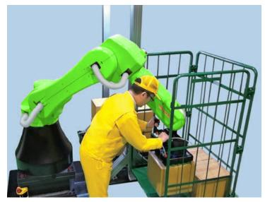
Workpiece transfer with Hand Guidance
