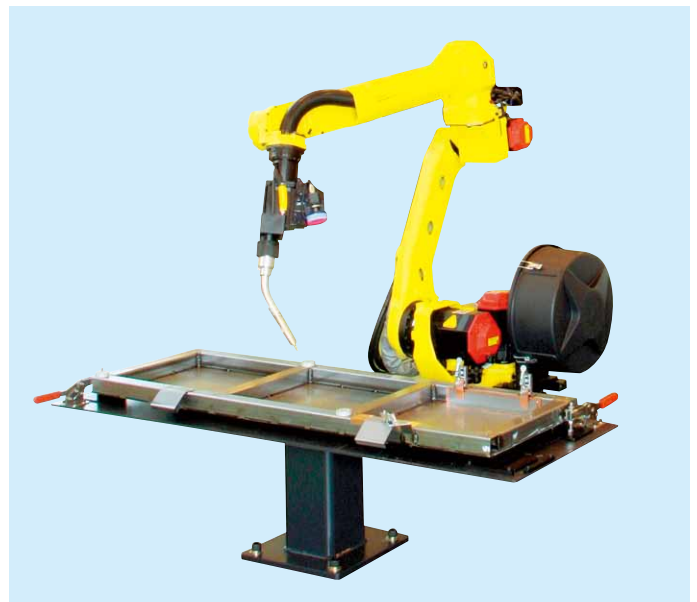
Architectural part arc welding with i RVision
