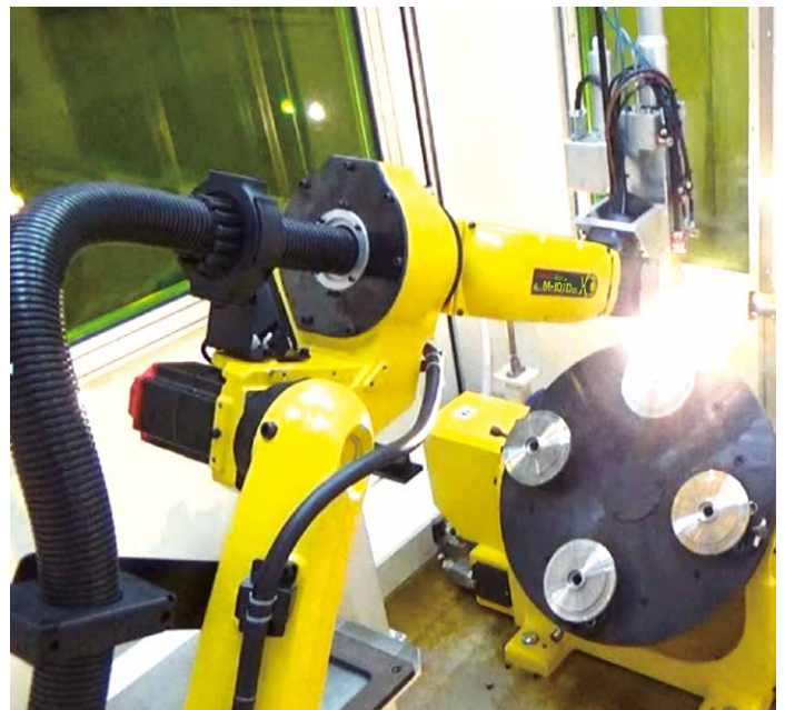
FIBER LASER welding
