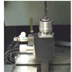
Tool length switch for automatic measurement
