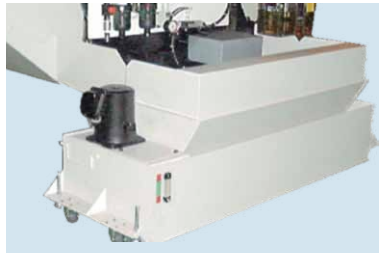
Coolant unit (tank)
