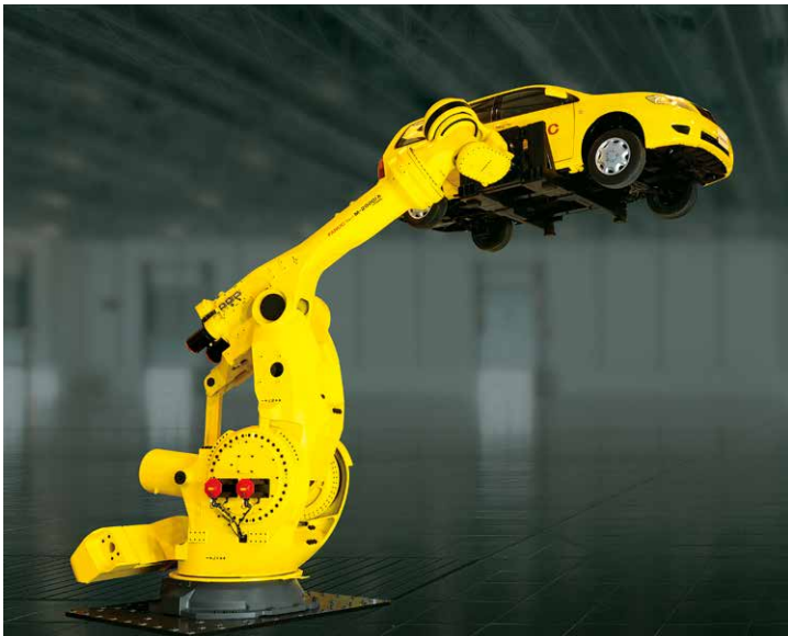
Completed car handling by M-2000iA/1700L
