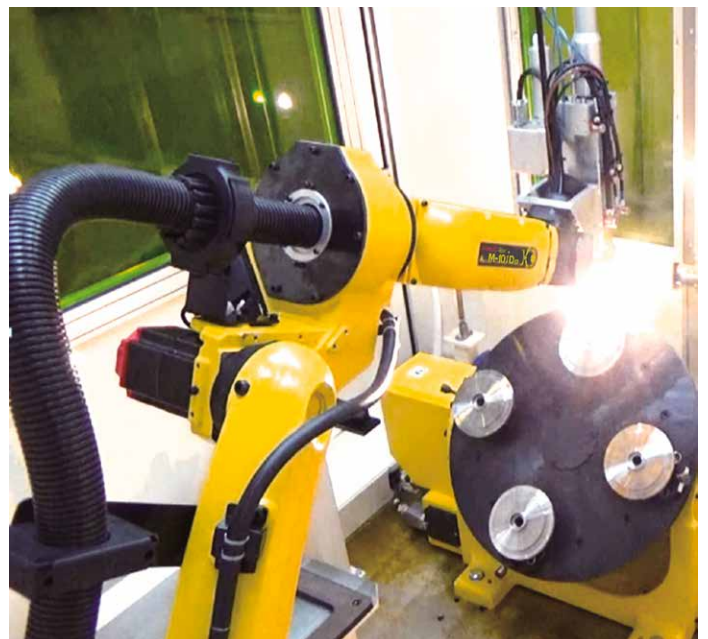
FIBER LASER welding
