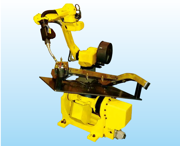
Automobile part arc welding with Servo Torch
